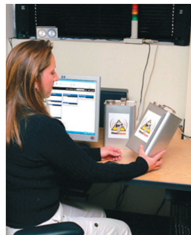
NASA labels its chemical containers with RFID tags to avoid dangerous combinations during storage and handling.
